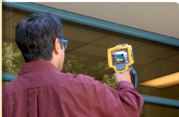
Roofing: Detect water-saturated insulation in flat-roof systems to locate damaged portions of roofing structure.
