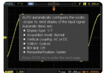
Built-in Help System Easy access to the Built-in help system by pressing and holding the key for 3 seconds
